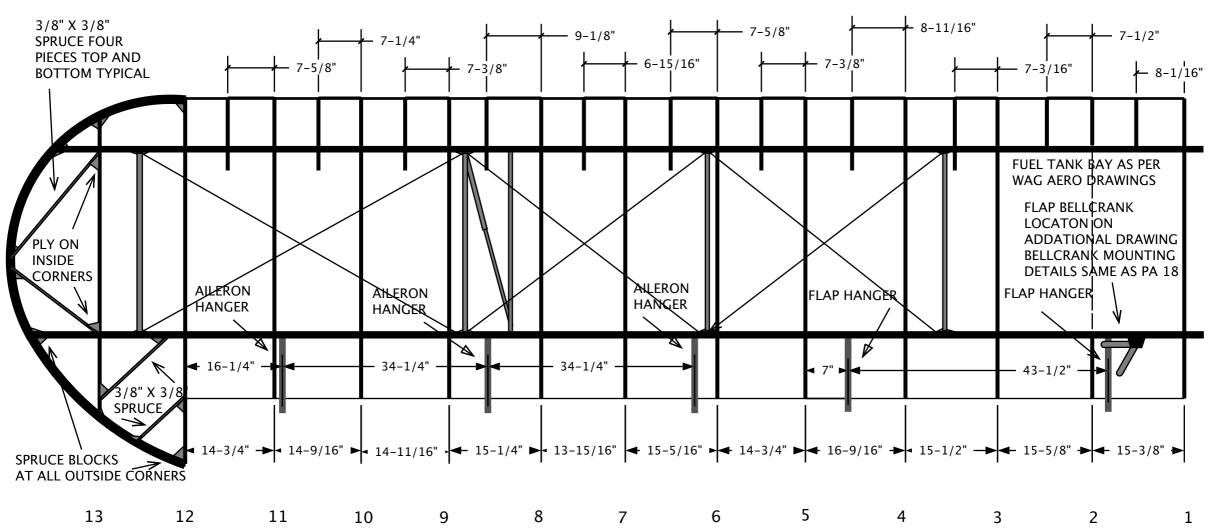
TIP RIB (#13) TO END OF REAR SPAR INSICE EDGE DIMENSION 11–3/16". TIP RIB TO END FRONT SPAR INSIDE EDGE 8–7/16".
